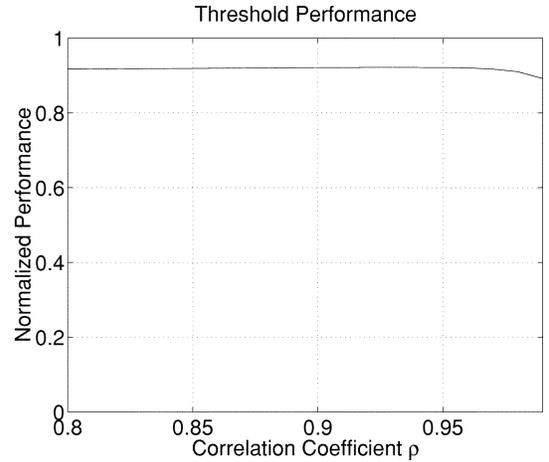
Fig. 4. Normalized performance of a threshold policy designed for a correlation coefficient of  $\rho = 0.95$ . The performance loss associated with this suboptimal scheme is minimal with a degradation of at most 10%.
