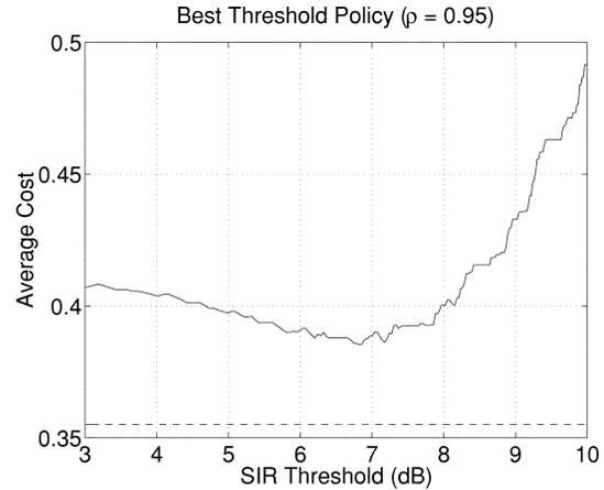
Fig. 3. Expected cost of threshold policies for various thresholds. The performance of the best threshold policy comes close to that of the optimal single-user policy.
