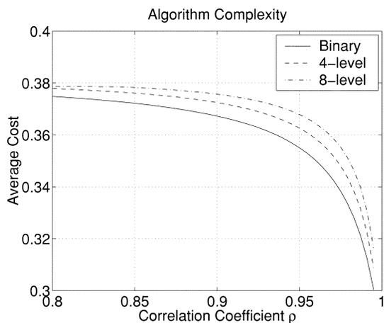
Fig. 5. Performance of algorithms with various complexity. For a fixed feedback bit rate, the optimal binary algorithms outperforms the more complex schemes.
