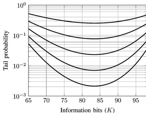
Fig. 5. Tail probabilities in the equilibrium packet distribution of the queue  $\Pr(Q > \tau)$ , for threshold values  $\tau \in \{5, 10, 15, 20, 25\}$ , as functions of the number of information bits  $K$  per codeword. The minimums occur uniformly at  $K = 83$  for all threshold values.
