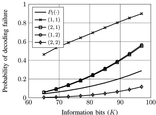
Fig. 3. Probability of decoding failure,  $P_f(N-K)$ , as a function of the number of information bits per codeword. The conditional probabilities of decoding failure for various values of  $(c_1, c_{N+1})$  are also included.
