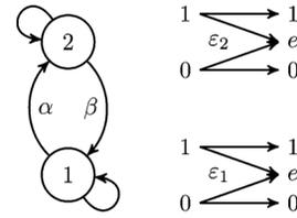
Fig. 1. Gilbert–Elliott bit erasure channel is employed to model the operation of a communication link with memory. This model captures both the uncertainty associated with transmitting bits over a noisy channel and the correlation over time typical of several communication channels.
