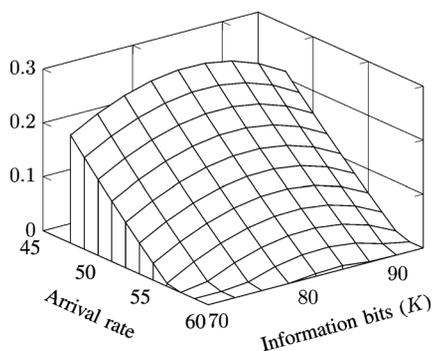
Fig. 6. Tail decay rate,  $-\lim_{\tau \rightarrow \infty} \frac{1}{\tau} \log \Pr(Q > \tau)$ , as a function of the number of information bits  $K$  per codeword and the average arrival rate  $\gamma \rho^{-1}$  in bits per codeword transmission interval.
